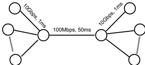
Figure 1. The network topology with simple bottleneck link.
